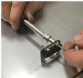
Figure 13 - M3 screws to secure magnet to the metal tab
