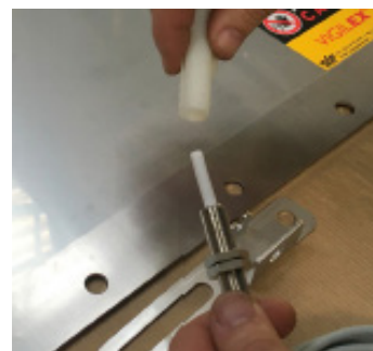
Figure 5 - Plastic cap removal
